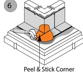
6. Remove half of the release liner from the Peel & Stick Corner and fold it in half with the tape side exposed. Center and mate the corner to the adhesive on the vertical surfaces. Reach between the folded layers of flashing and press the upper flap into the point of the corner, using the sides of your hands. Pull, tightly flare and stretch the flashing into the angle change onto the horizontal surface. Avoid bridging and gaps. Hand Roll.
