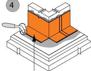
4. Align edge of the Peel & Stick flashing or flashing membrane with the Seam Tape, leaving 1/4" of the tape exposed. Press the flashing into the angle change to minimize bridging, and continue up the vertical. Hand roll. Continuously wrap flashing around curb and cut corners to fit square with the curb.
