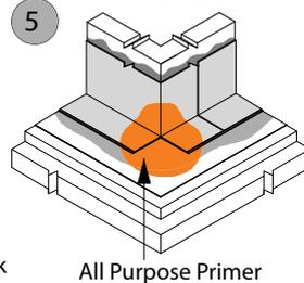
4. Align edge of the Peel & Stick flashing or flashing membrane with the Seam Tape, leaving 1/4" of the tape exposed. Press the flashing into the angle change to minimize bridging, and continue up the vertical. Hand roll. Continuously wrap flashing around curb and cut corners to fit square with the curb.
