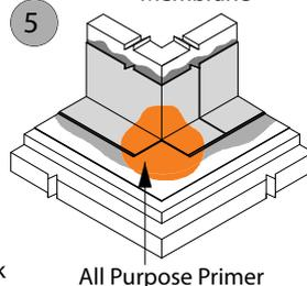
5. Apply All Purpose Primer to the corner flashing area. Allow to flash off.
